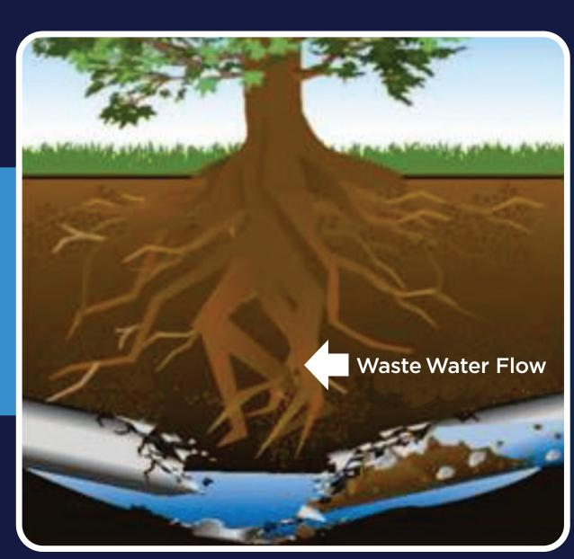
The pipe cannot withstand the downward pressure of the earth where the pipe is not properly supported, leading to total collapse. The pipe needs to be replaced with elevation changes allowing for properly supported, downward pitch.
