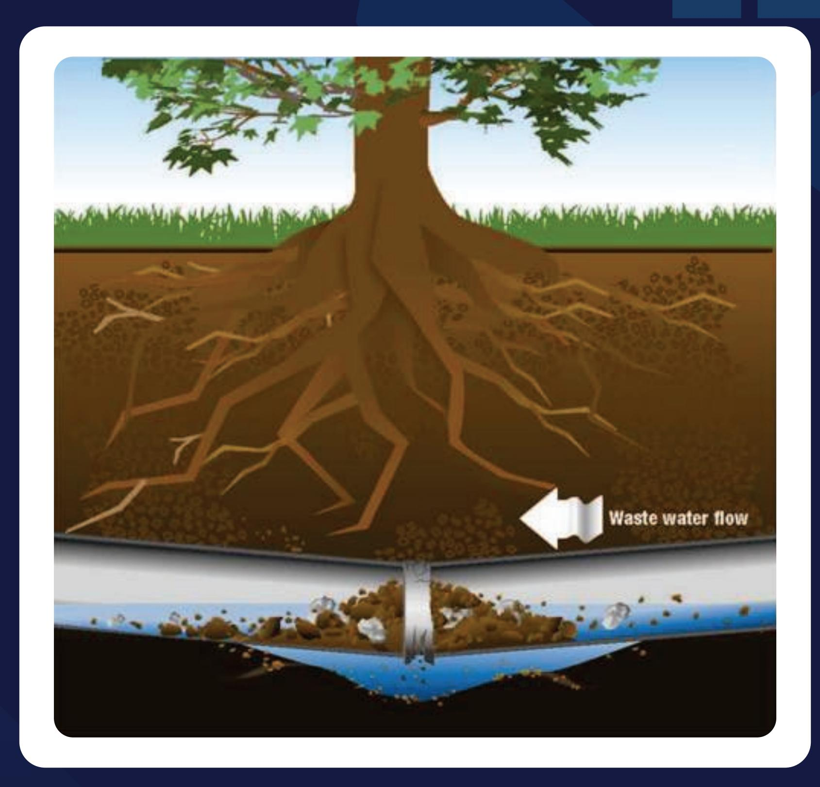
Pipe bellies usually occur due to improper installation where the pipe is not adequately pitched downward.
