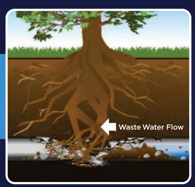
The roots have compromised the pipe's integrity, and the pipe is beyond rehabilitation. Pipe replacement is typically needed.
