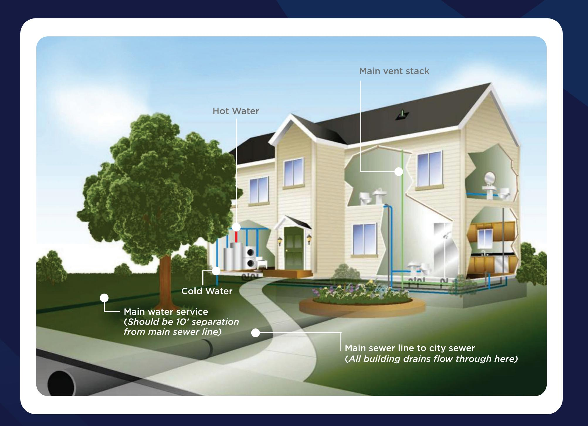
Water enters the house through the main water service line and is distributed to each fixture.
