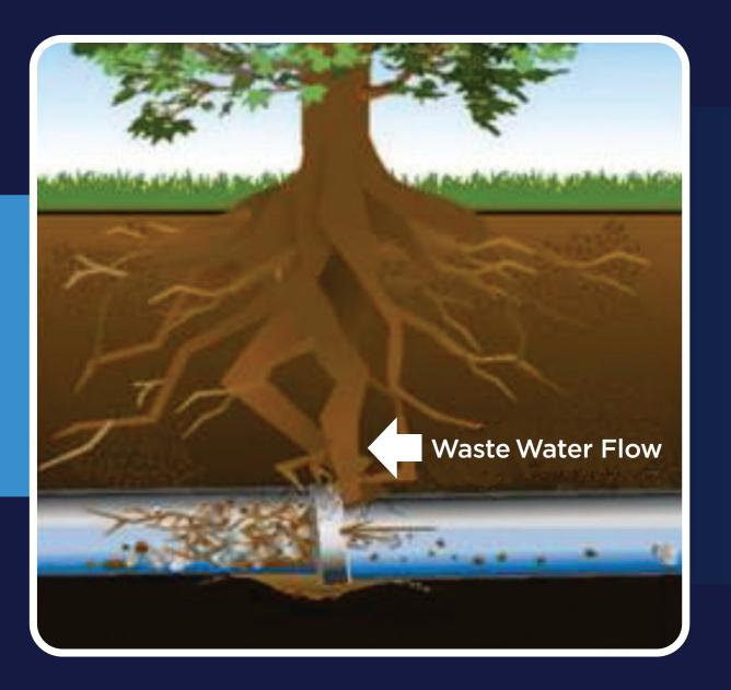
Roots overtake the pipe, choking off the sewer line flow and causing partial or complete blockages. There is usually still an opportunity to rehabilitate the existing line.
