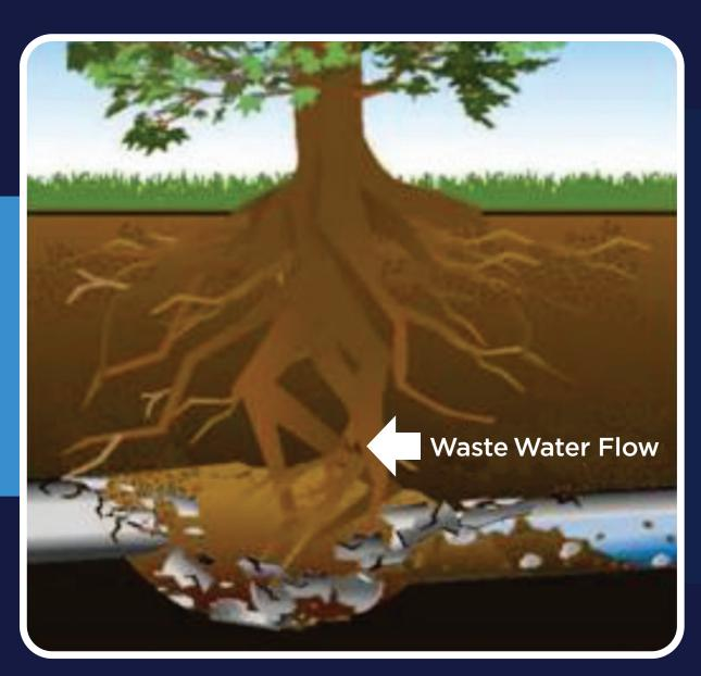
The foundation for supporting the pipe is completely compromised, and the weight of the earth collapses the pipe completely.
