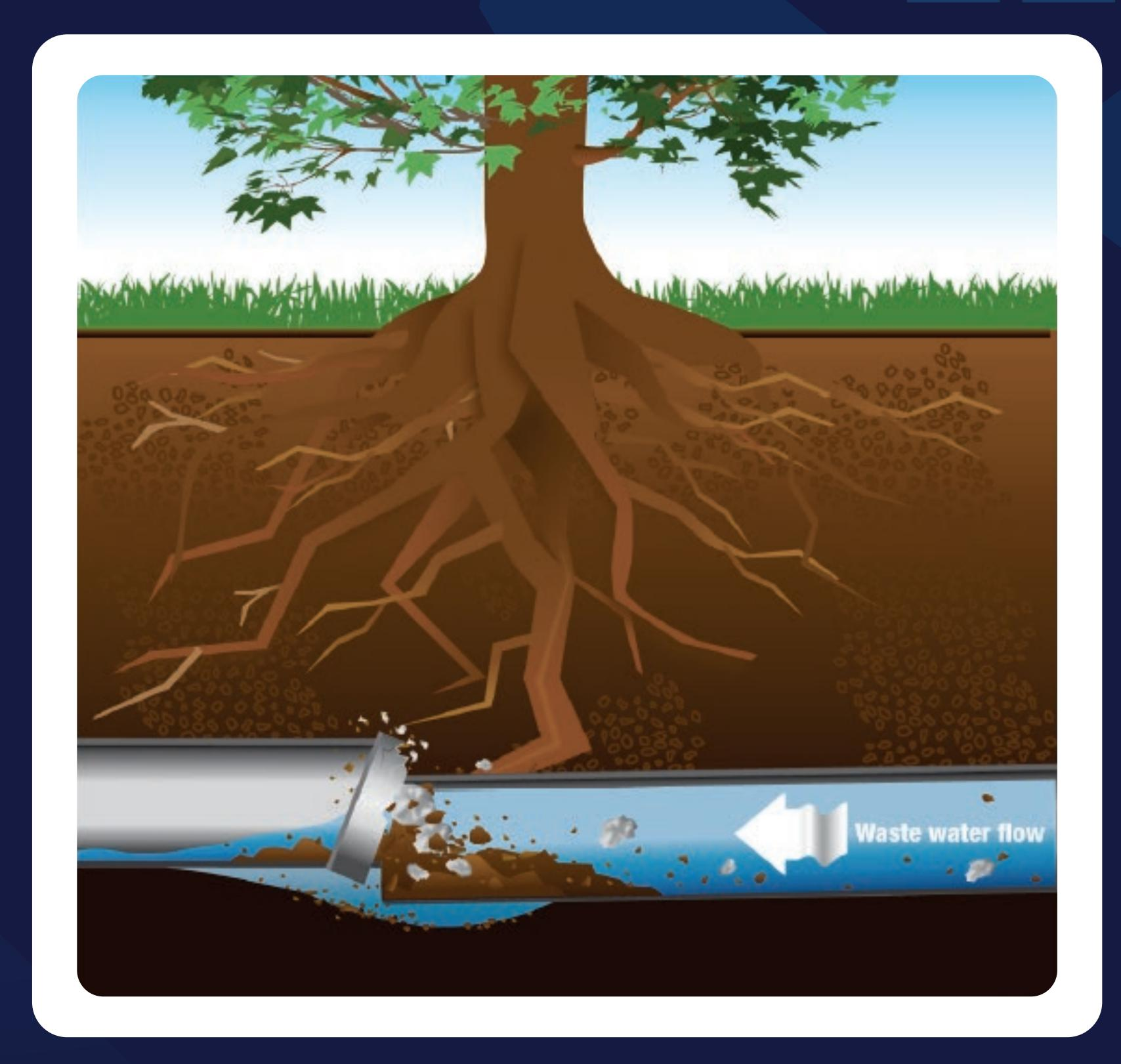
Pipe misalignment can occur due to improper installation. Insufficient gravel bedding can cause the pipe to shift from ground settling. As the pipe shifts, water begins to leak out and erode the earth beneath the pipe.
