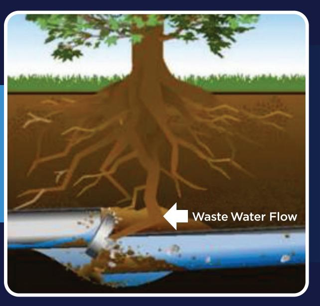
The void beneath the pipe grows larger due to wastewater erosion, and the pipe loses its natural support.
