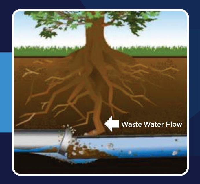
Normal settling of the ground causes the pipe to shift slightly, and wastewater begins to leak outside of the pipe.
