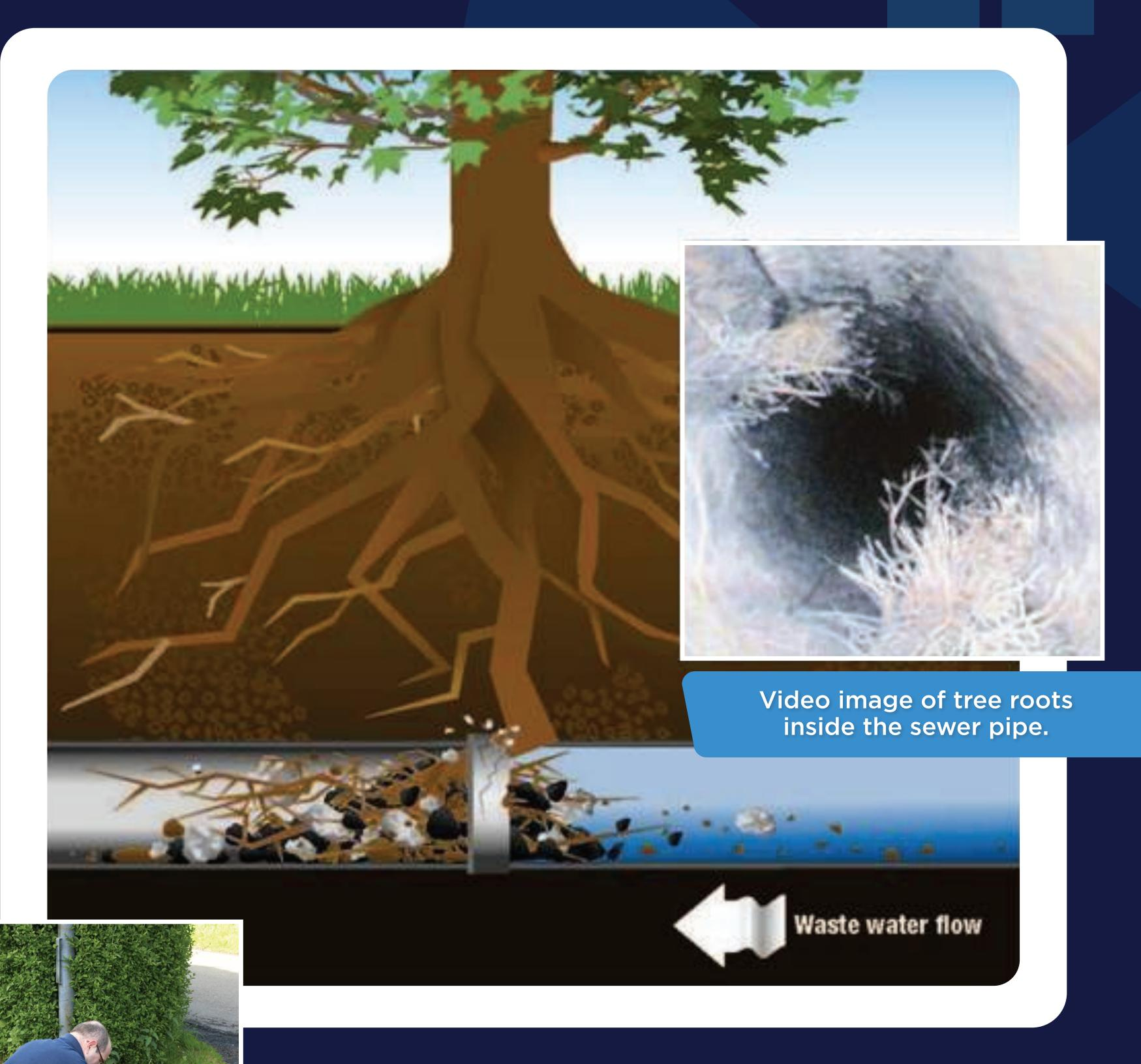
Tree roots are a common culprit for main sewer stoppages, especially in homes that were built before 1970. Due to the ground settling over time, the pipes can shift enough to break the mortar seal at pipe connections, allowing moisture-seeking roots to penetrate the sewer line. Once the seal is broken, the roots gravitate to this water and nutrient-rich source, eventually overtaking the pipe.
